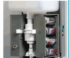
3. Install the batteries
